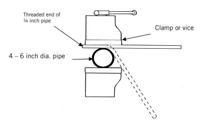
Figure 3: Pipe bending using a clamp or vice
