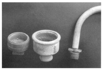
Figure 5: Separate components of the mercury retort
